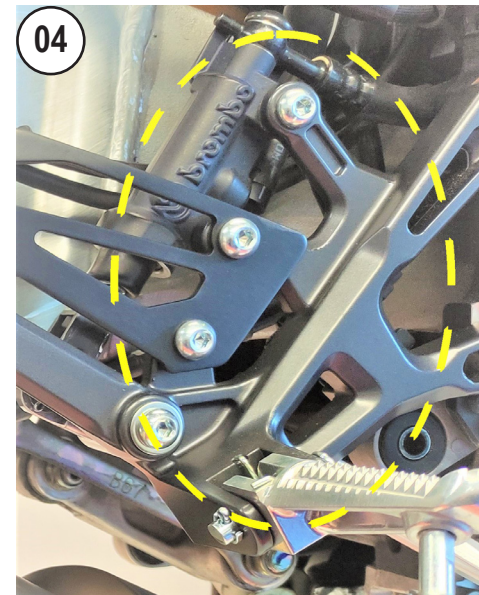
SECURE THE CABLES TO A POINT NOT INTERFERING WITH MOVABLE AND/OR HOT PARTS OF THE MOTORCYCLE
