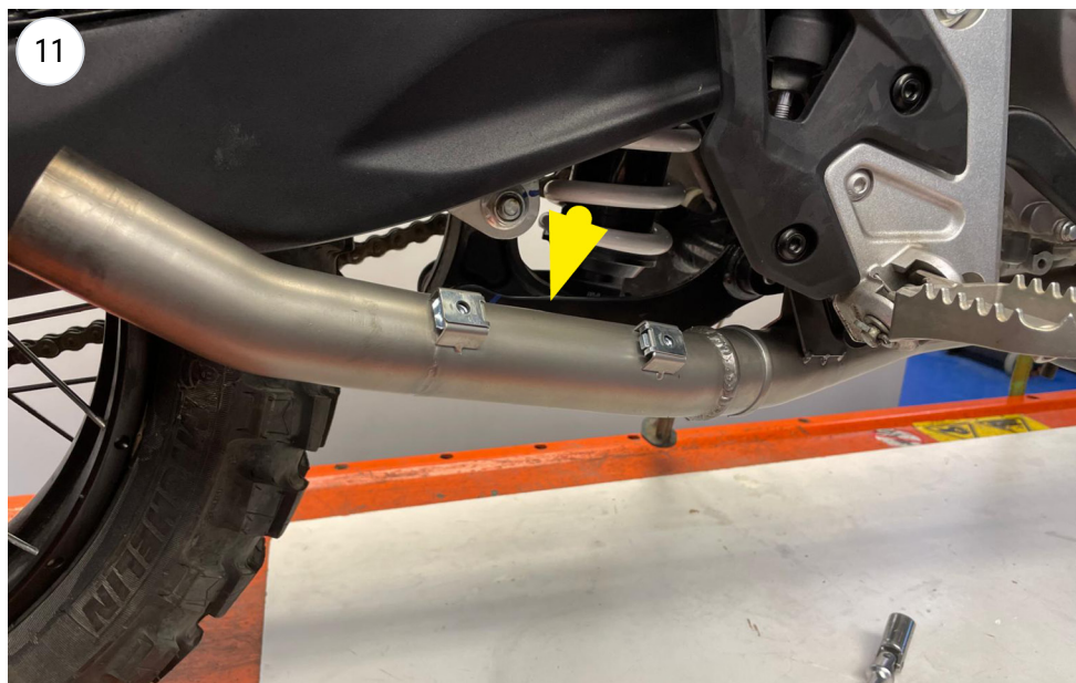
fit the final pipe
