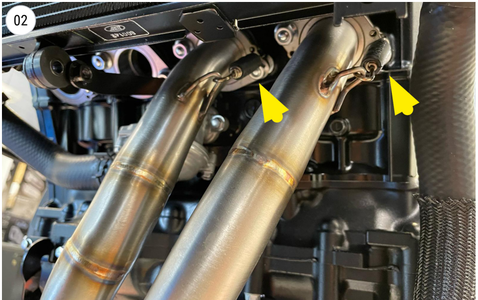
install primary pipes
