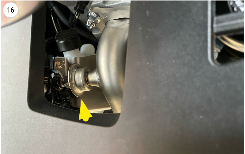
reinstall the Lambda/Oxygen sensor
