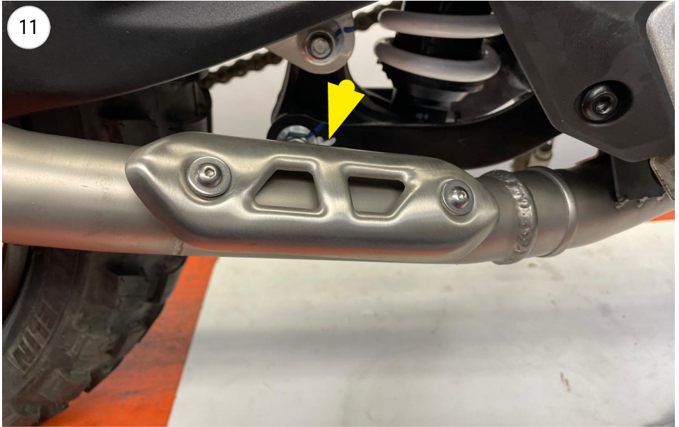
install the heat shield
