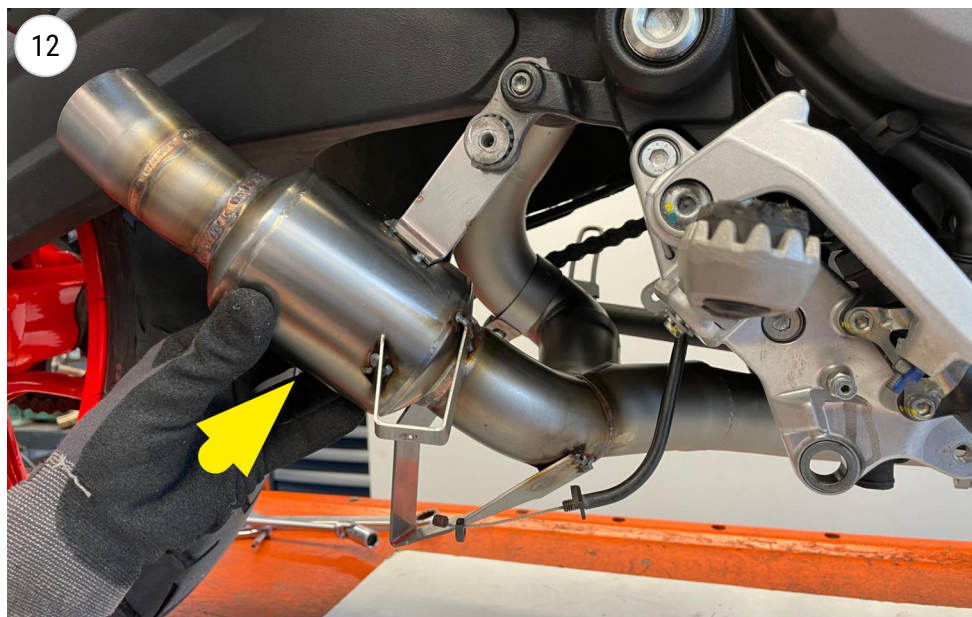
Install the pipe
