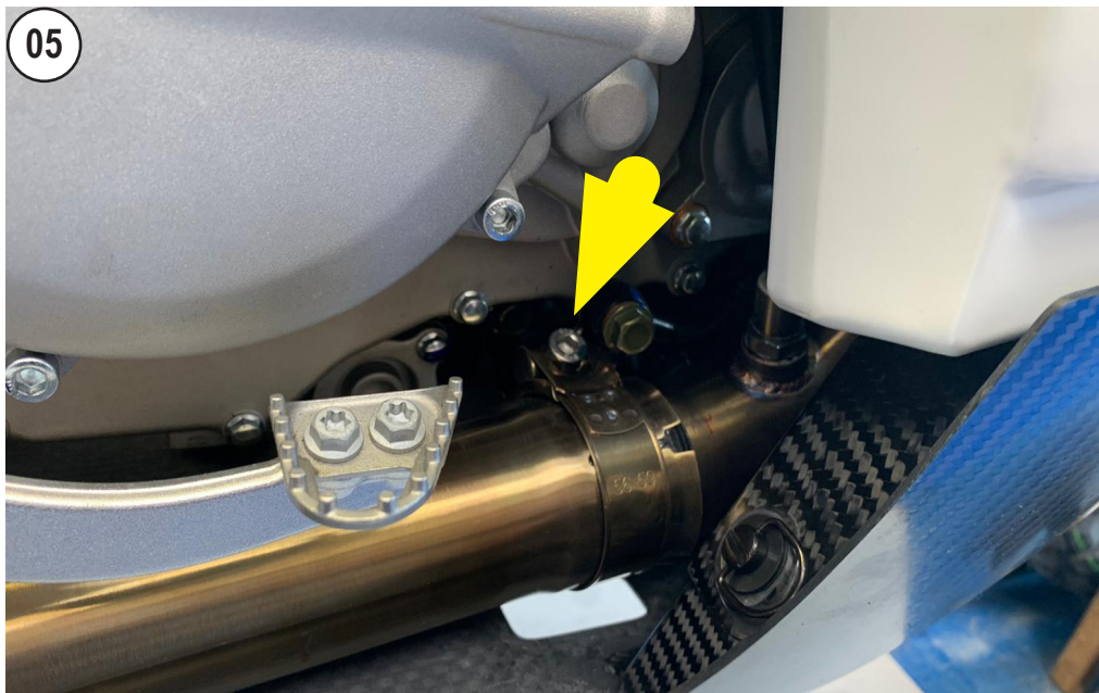
LOOSE THE CLAMP AND REMOVE THE STOCK PIPE
