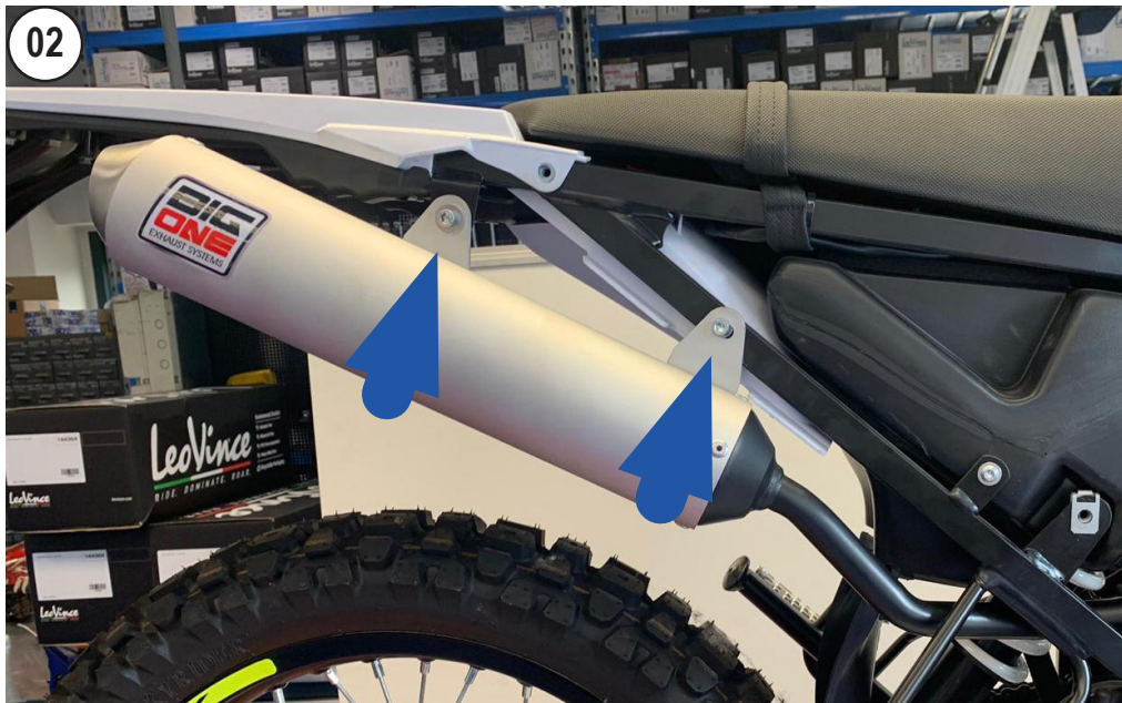
UNSCREW AND REMOVE THE MUFFLER
