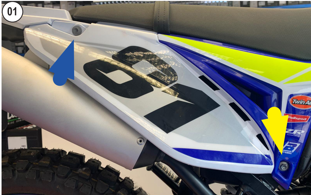
UNSCREW AND REMOVE THE SIDE PANEL
