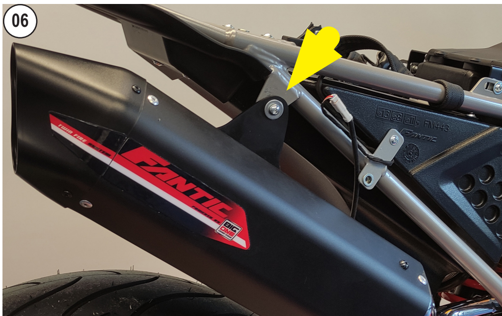
UNSCREW AND REMOVE THE MUFFLER
