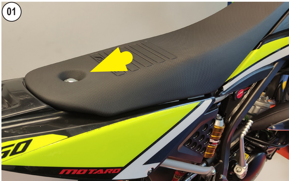
UNSCREW AND REMOVE THE DRIVER SEAT
