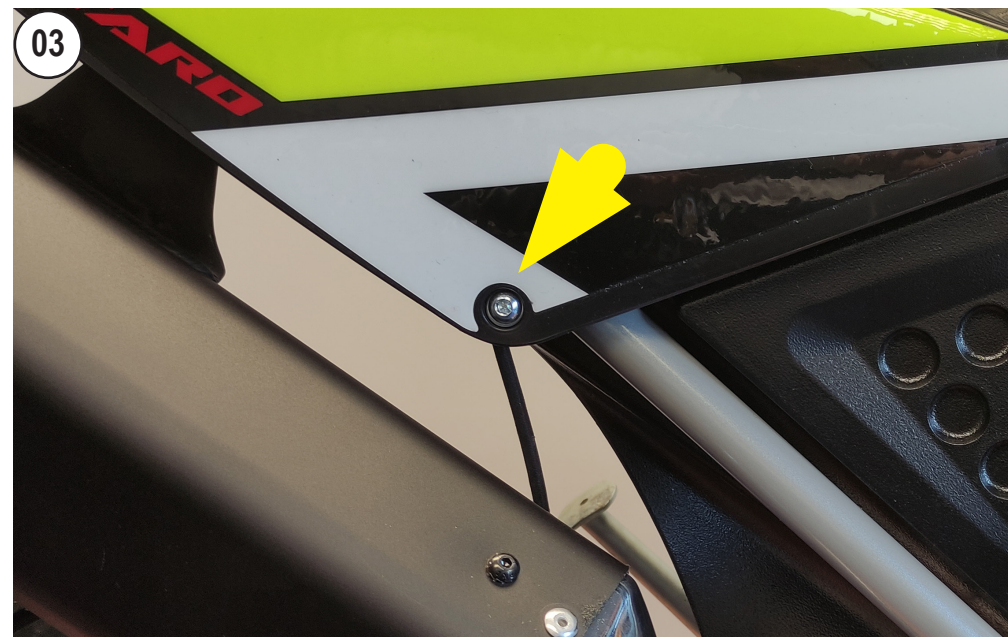
UNSCREW AND REMOVE THE SIDE PANEL
