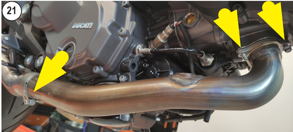
INSTALL THE FRONT PRIMARY PIPE
