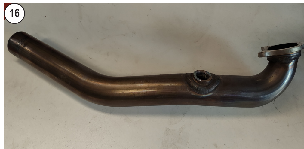
REMOVE THE FRONT PRIMARY PIPE
