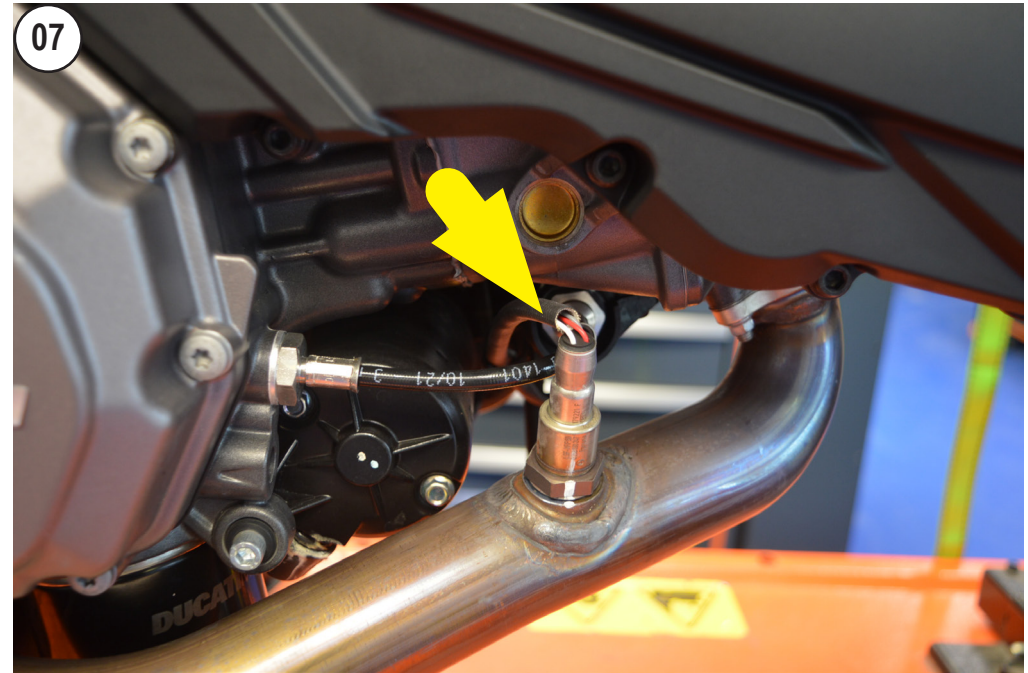
REMOVE THE LAMBDA SENSOR
