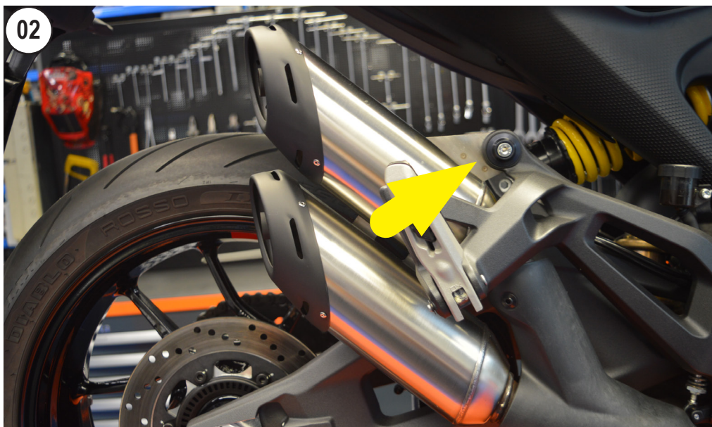
UNSCREW - REMOVE THE FASTENERS (Ducati Monster 937)
