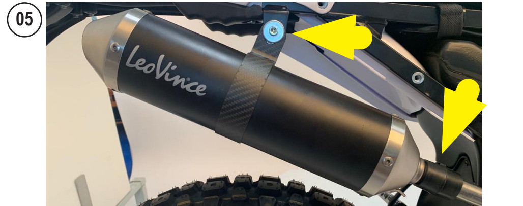
INSTALL THE LV MUFFLER - REMEMBER THE RUBBER SLEEVE
