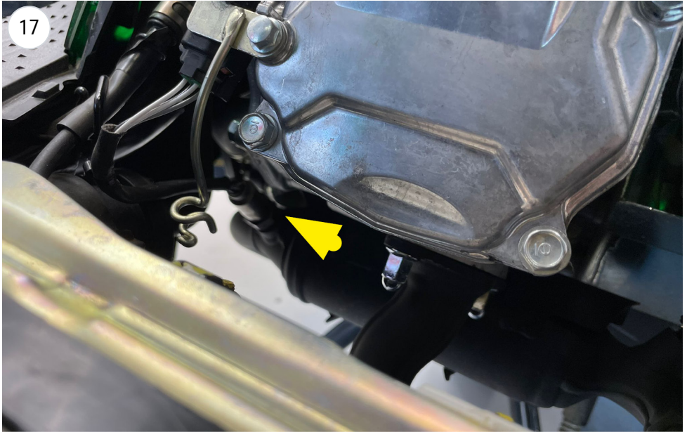
screw the Sonda lambda / O2 Sensor
