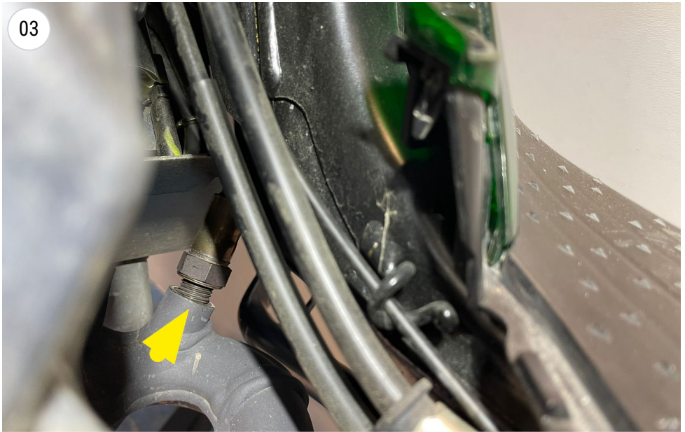
unscrew the Sonda lambda / O2 Sensor
