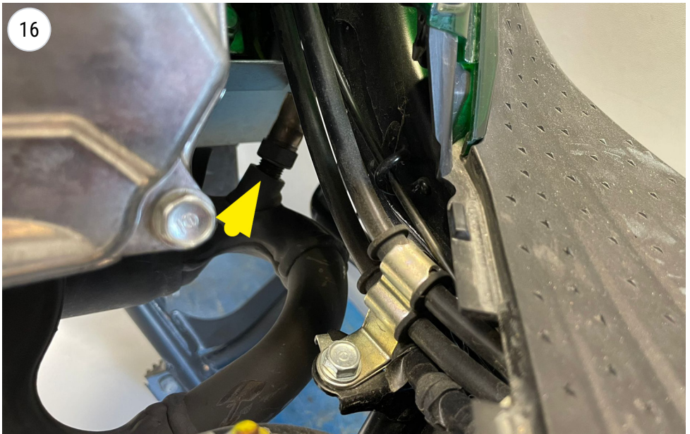
screw the Sonda lambda / O2 Sensor
