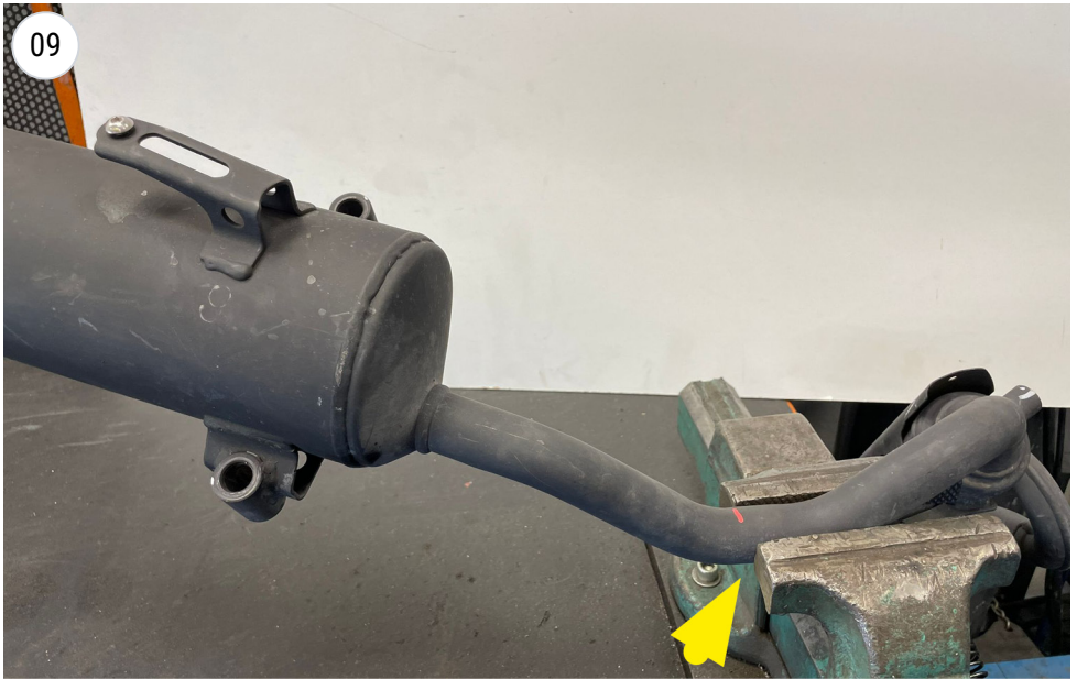
secure the exhaust in a bench vice
