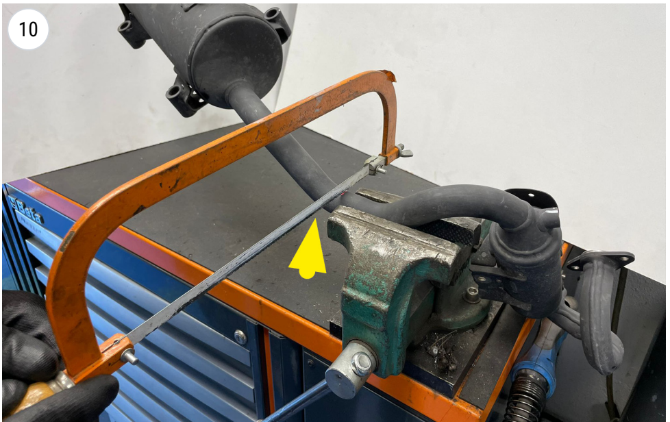
make the cut using a manual hacksaw, not an angle grinder
