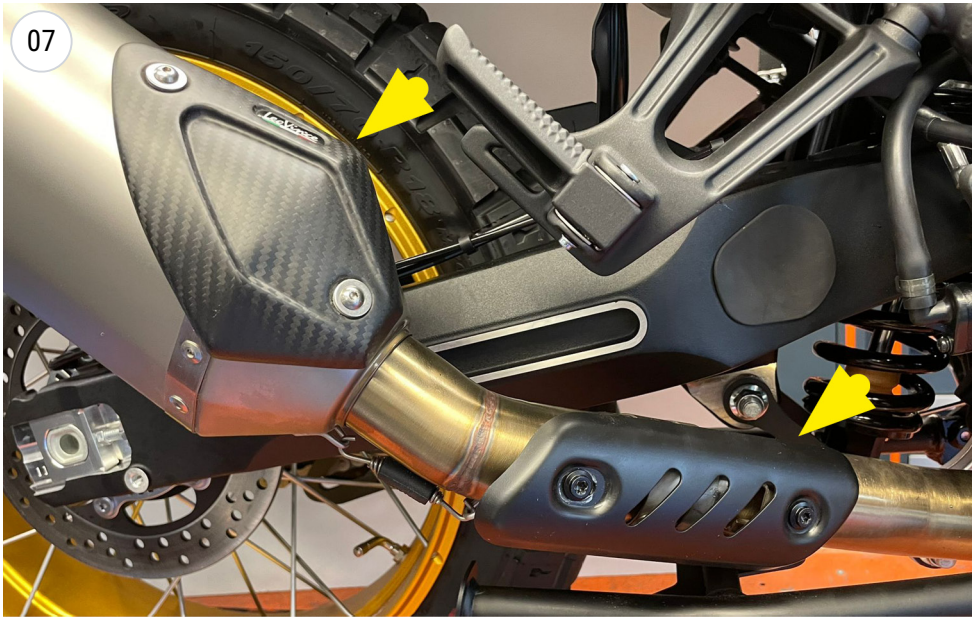
fit the heat shields
