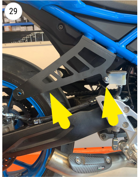
29 FIT THE LEOVINCE BRACKET AND FIT THE BRAKE OIL PAN
