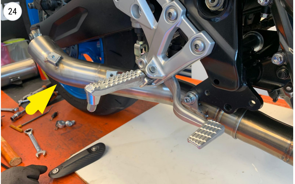
INSTALL THE FINAL PIPE
