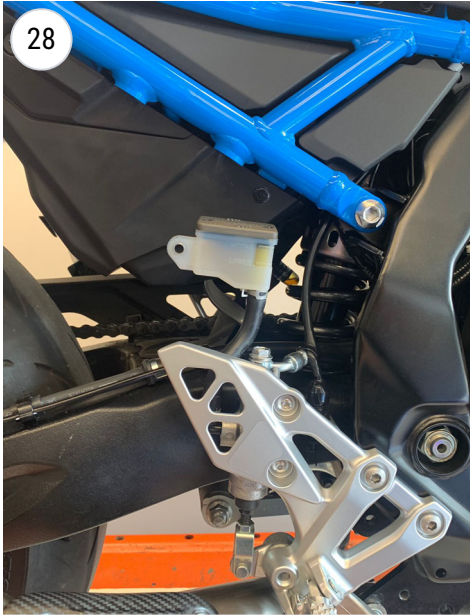
28 REMOVE THE STOCK PASSENGER FOOTPEG
