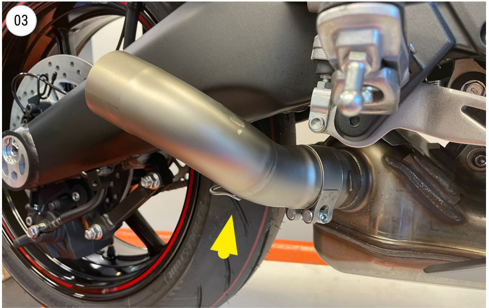
INSTALL THE LEOVINCE PIPE
