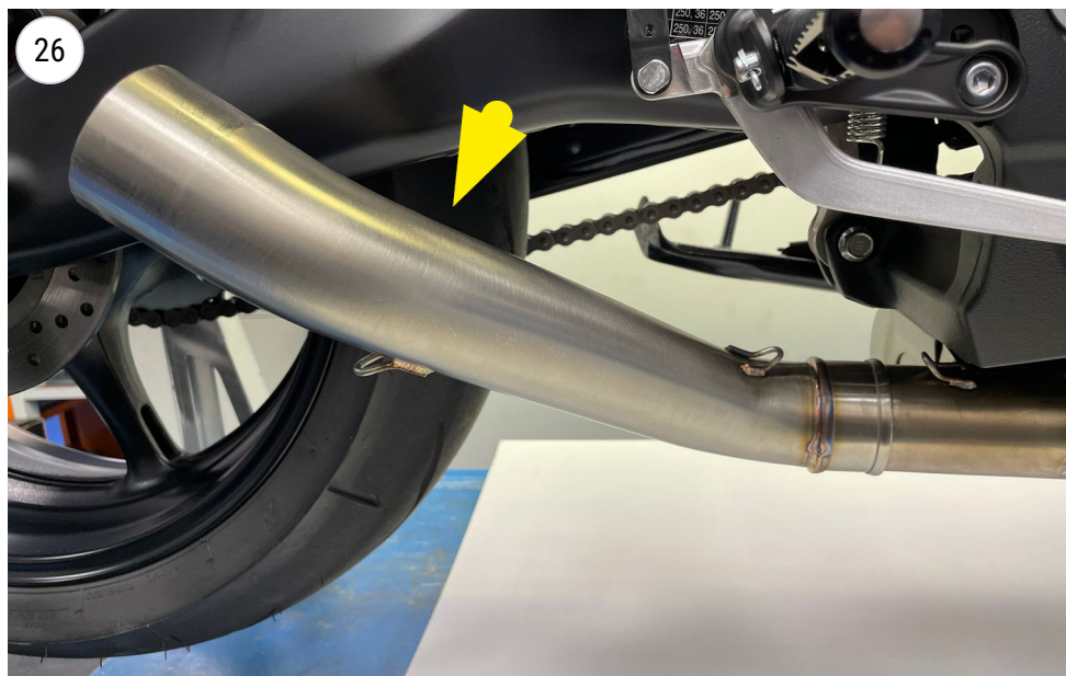
fit the final pipe
