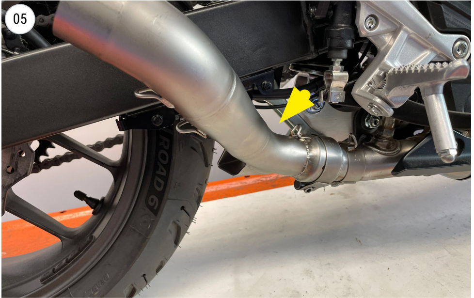
fit the pipe with the clamp
