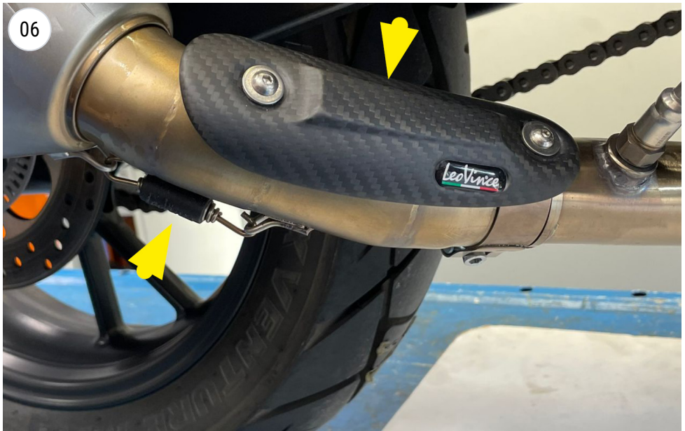
install the carbon heat shield and hang the spring
