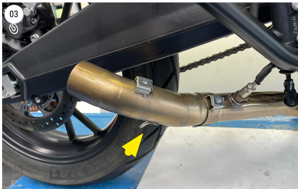
install the pipe
