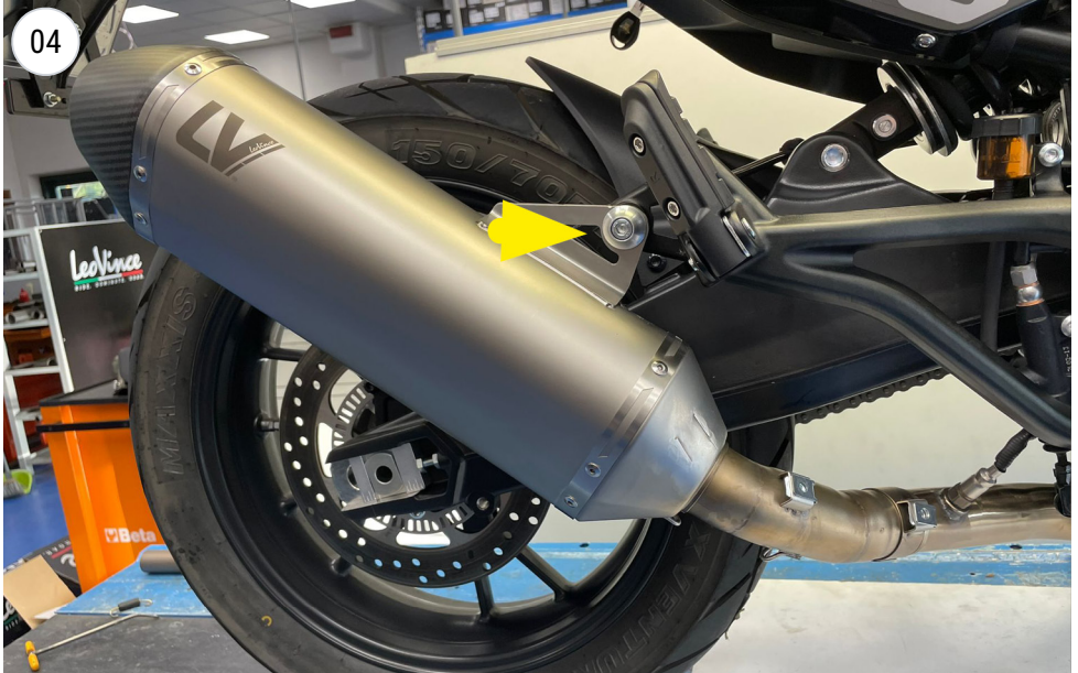
install the muffler
