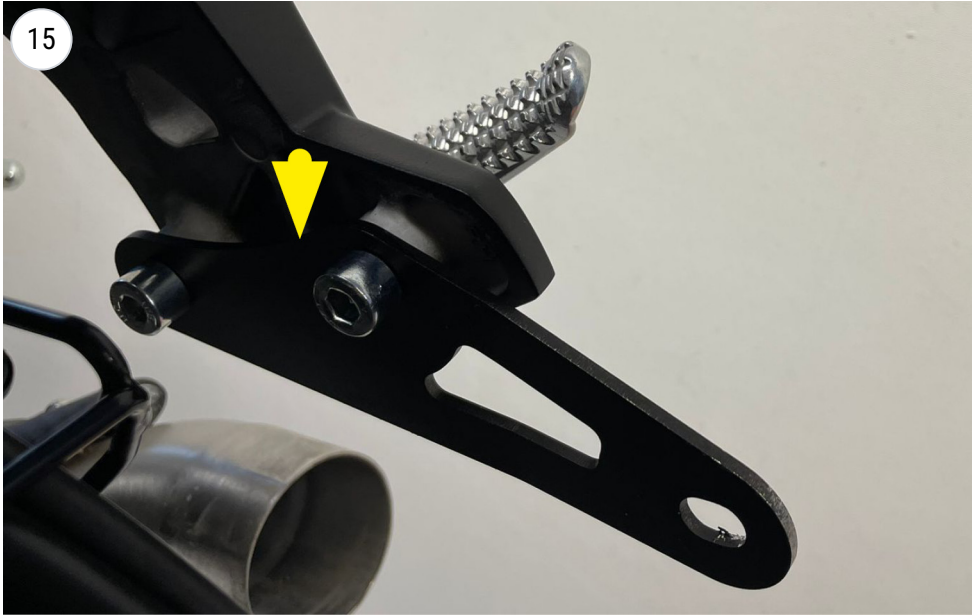
fit the bracket - ONLY ON YAMAHA TRACER 7
