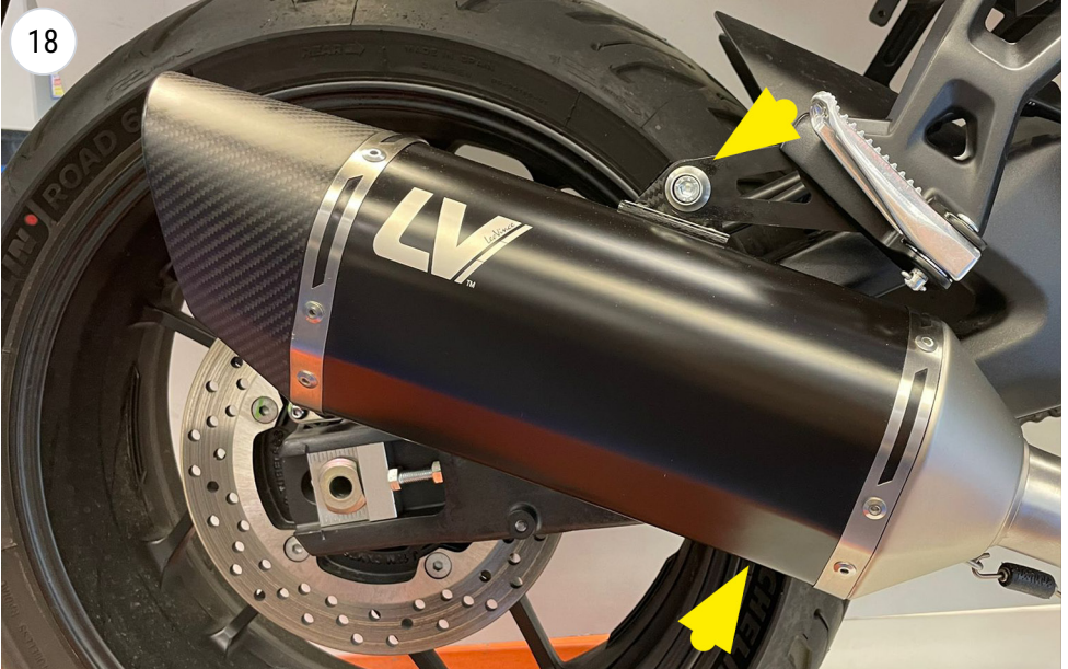
install the muller - ONLY ON YAMAHA TRACER 7
