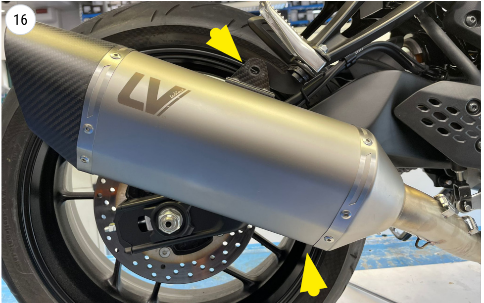
install the muffler - ONLY ON YAMAHA MT-07
