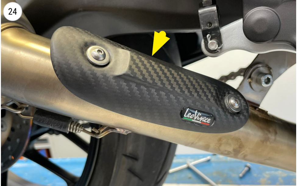
fit the carbon heat shield
