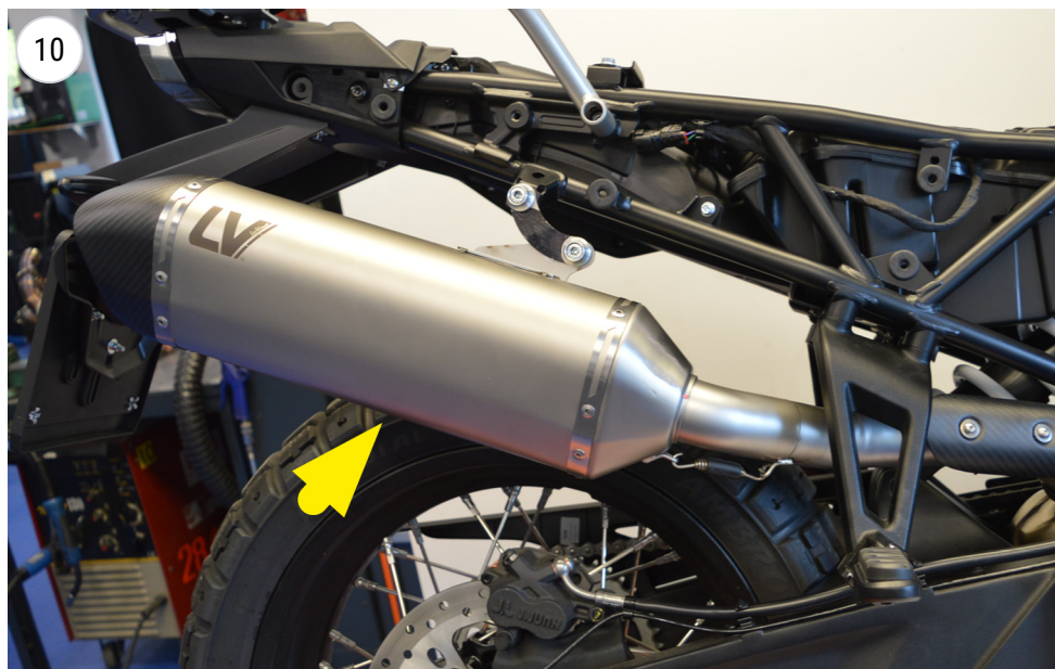
install the muffler (CF MOTO MT-X 800)
