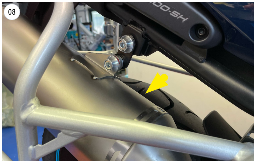
install the muffler (CF MOTO MT 800)
