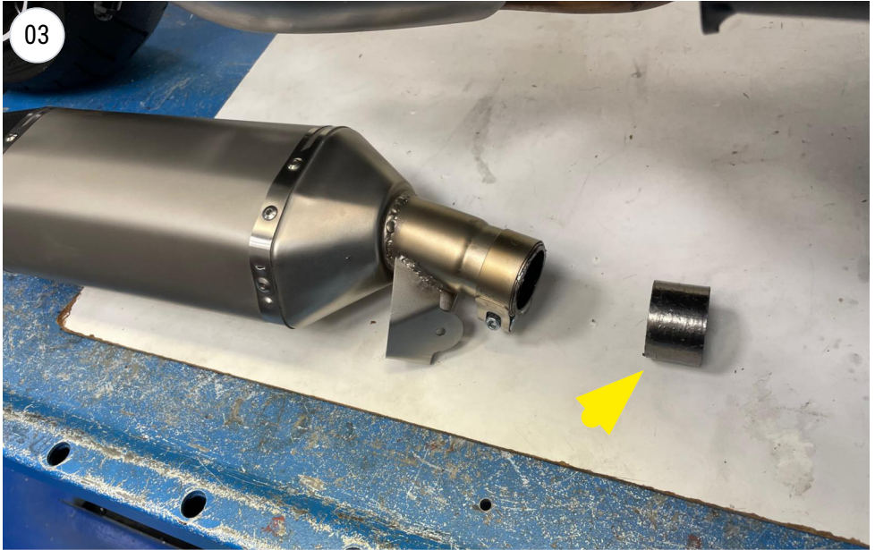
reinstall the stock bushing on LeoVince muffler
