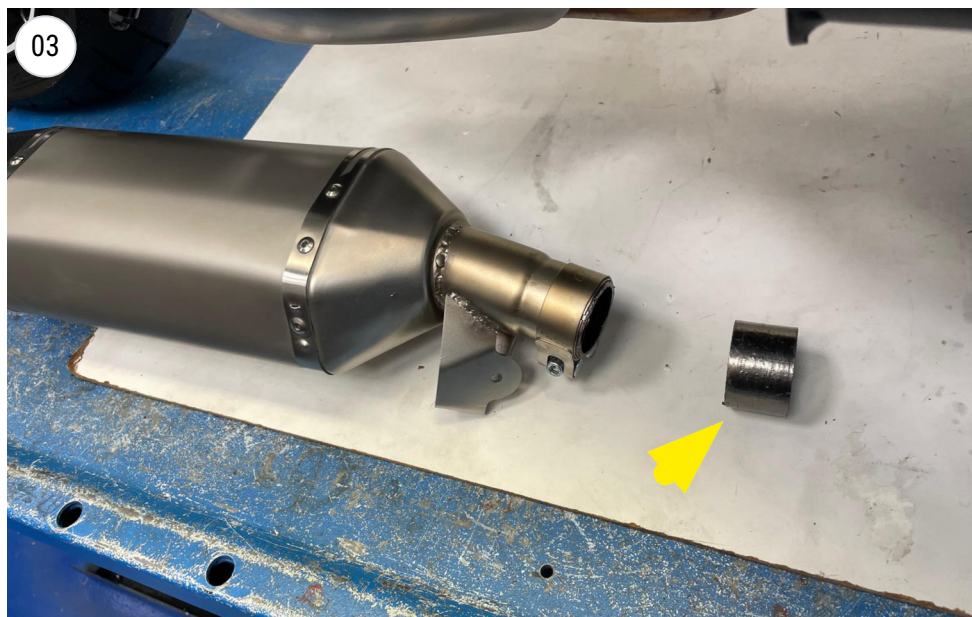
reinstall the stock bushing on LeoVince muffler
