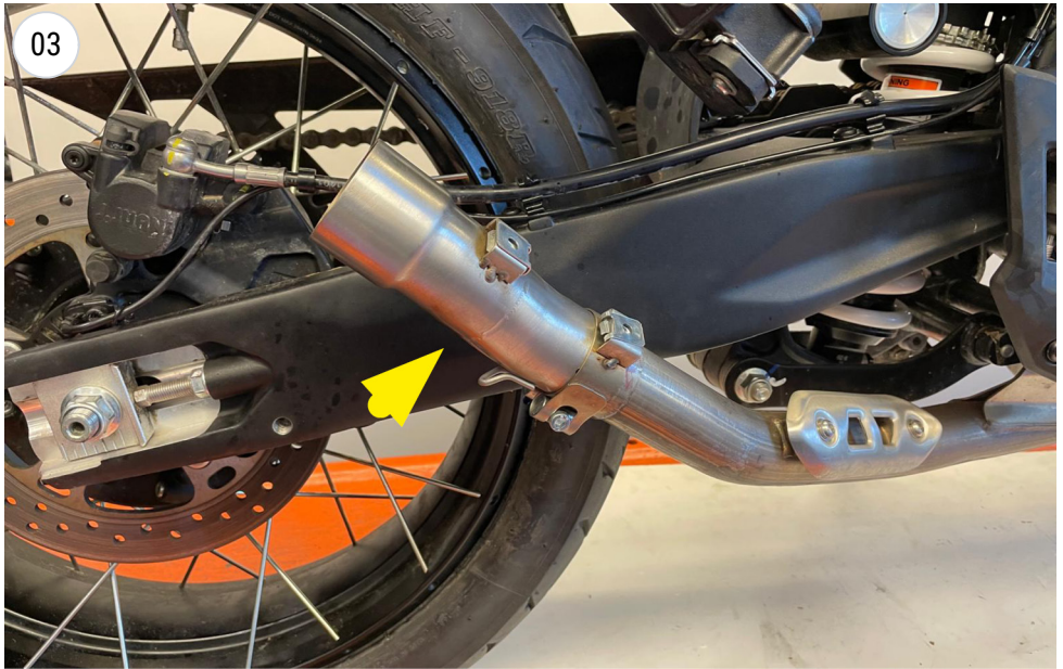
install the pipe with the clamp
