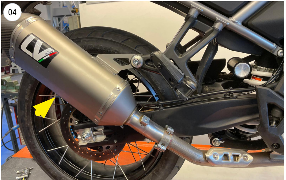
fit the muffler
