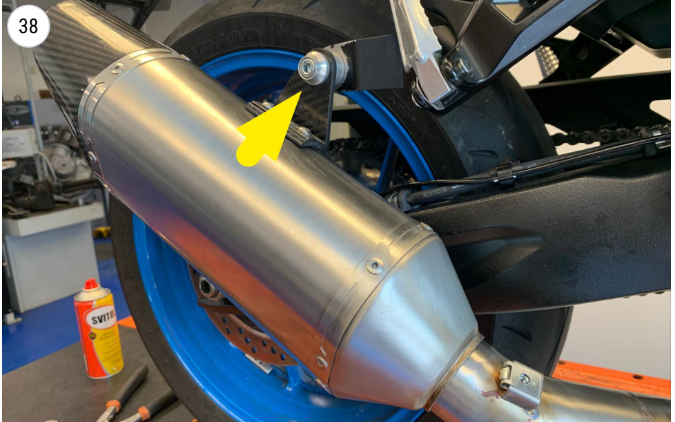
INSTALL THE MUFFLER - IF YOU HAVE THE OPTIONAL 80050 KIT GO ON PHOTO
