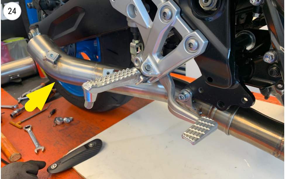
INSTALL THE FINAL PIPE
