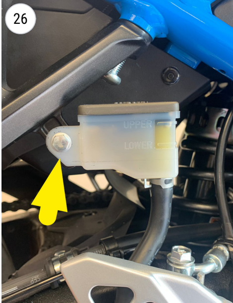
REMOVE THE BRAKE OIL PAN - ONLY IF YOU HAVE THE OPTIONAL 80050 KIT, OTHERWISE GO ON PHOTO 32
