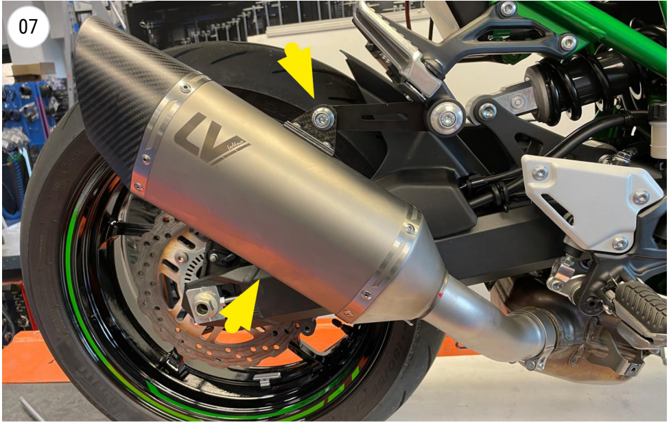
install the muffer
