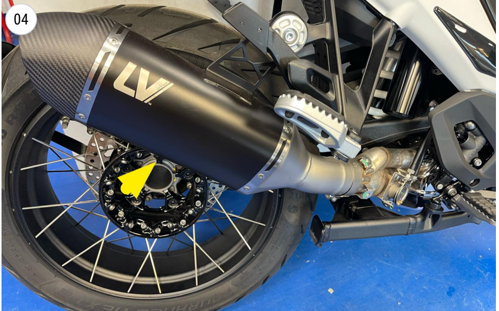
INSTALL THE MUFFLER
