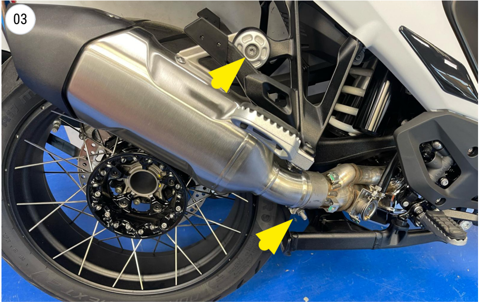
UNSCREW AND REMOVE THE MUFFLER
