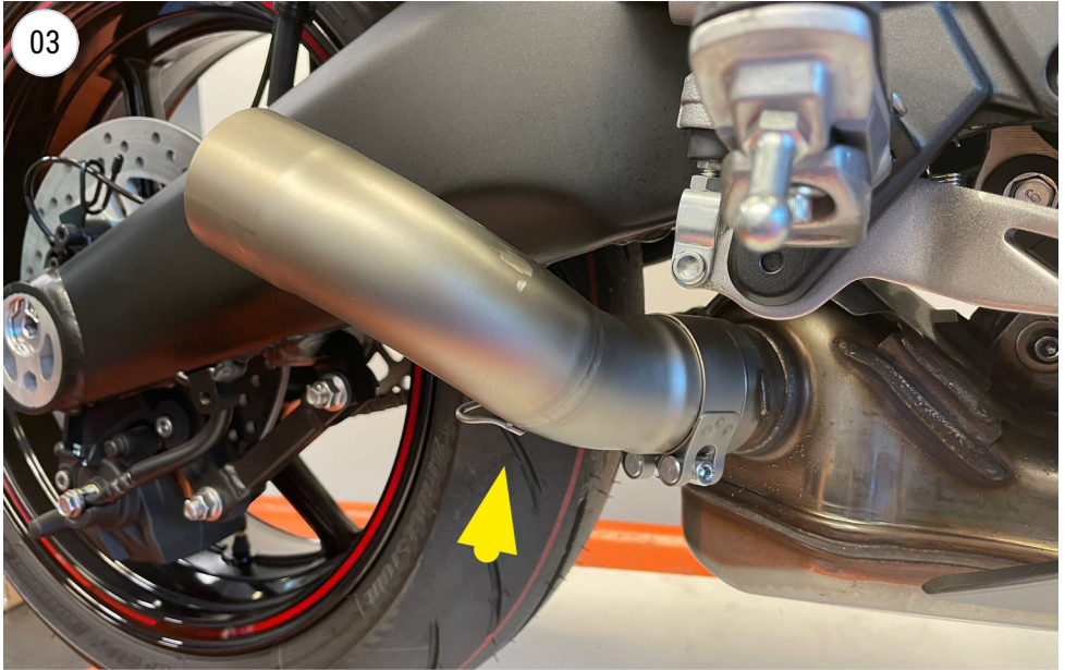
INSTALL THE LEOVINCE PIPE
