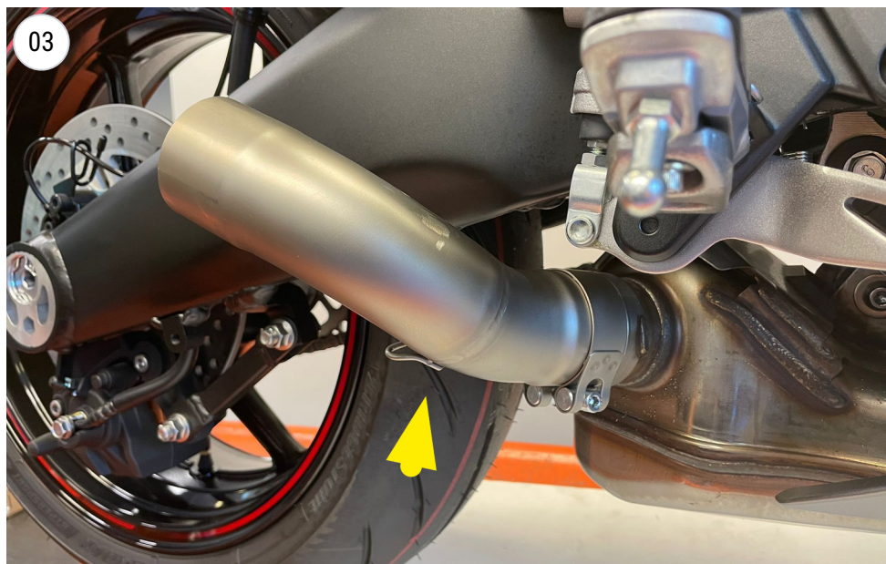
INSTALL THE LEOVINCE PIPE
