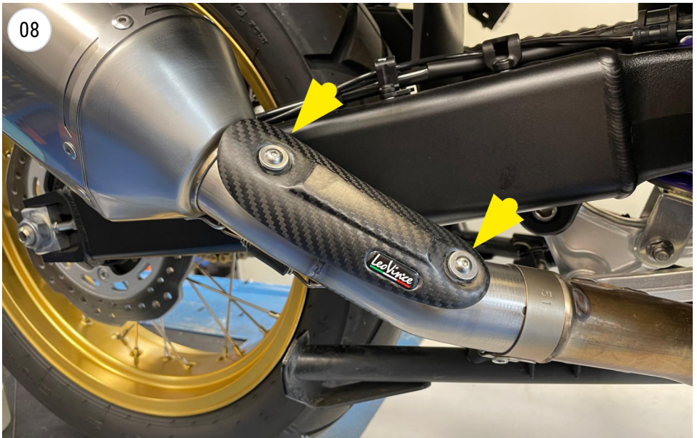
FIT THE CARBON HEAT SHIELD
