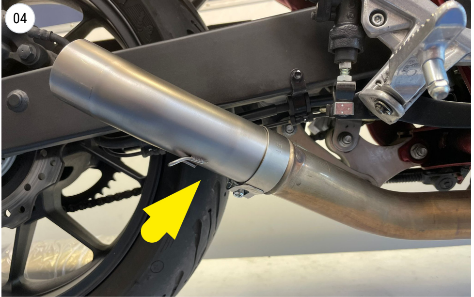
Install the pipe with the clamp
