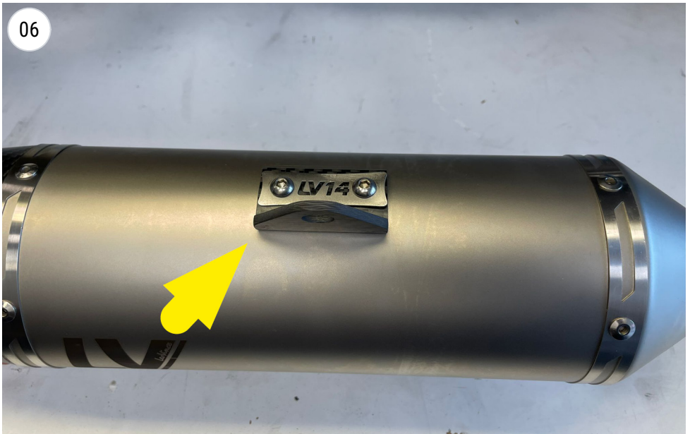
Fit the bracket on the muffler
