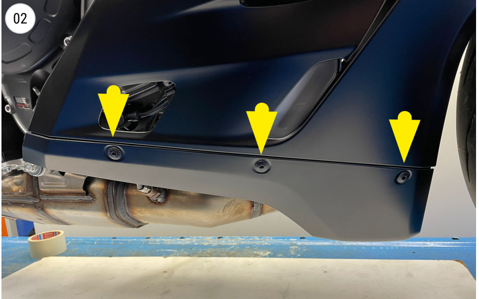
remove the plastic fasteners
