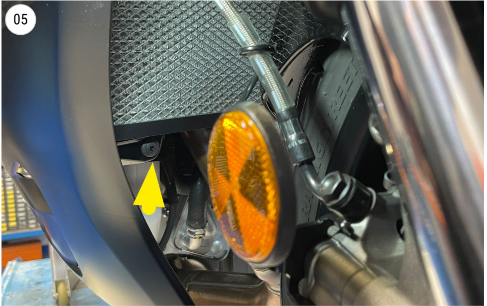
remove the plastic fasteners
