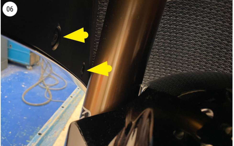
remove the plastic fasteners and remove the fairing
