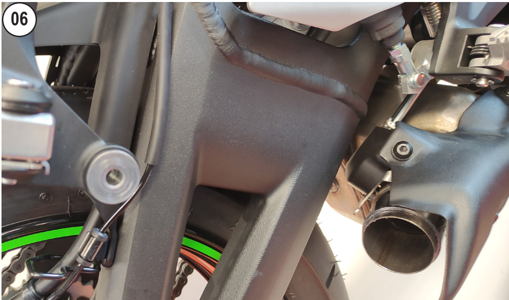
REMOVE THE FINAL PIPE
