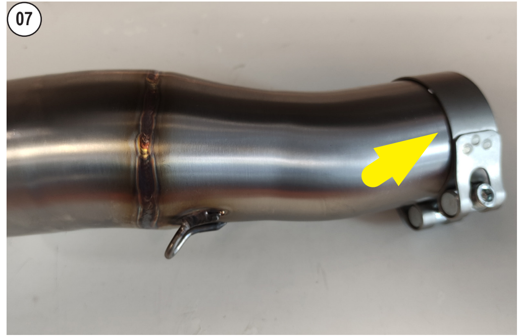
SLIP THE CLAMP ON THE PIPE
