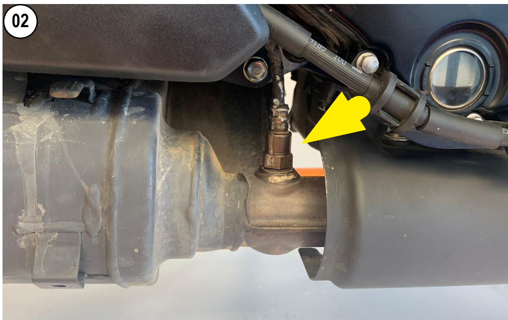
UNSCREW AND REMOVE THE LAMBDA SENSOR
