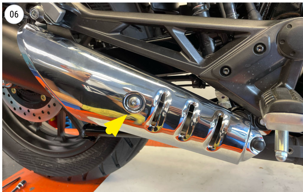
re-install the stock heat shield
