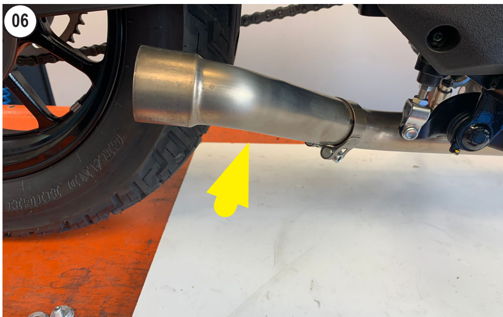
INSTALL THE LeoVince PIPE WITH THE LeoVince CLAMP
