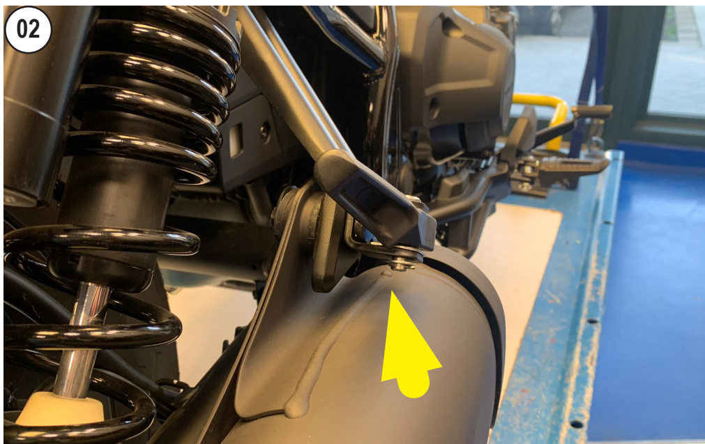
REMOVE THE FOOTPEG WITH ITS SUPPORT
