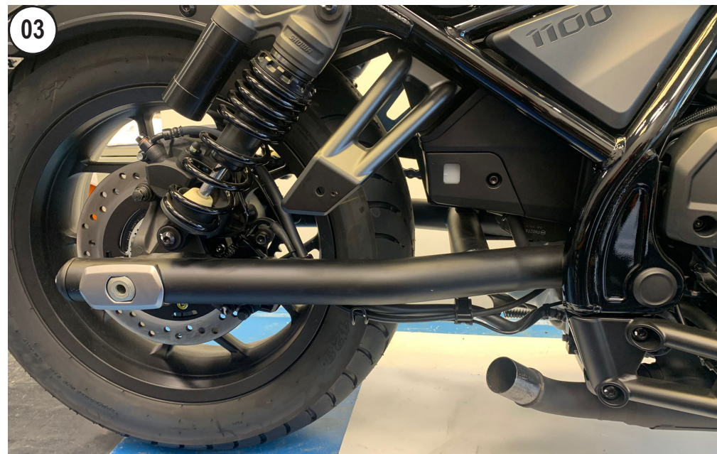
REMOVE THE STOCK MUFFLER
