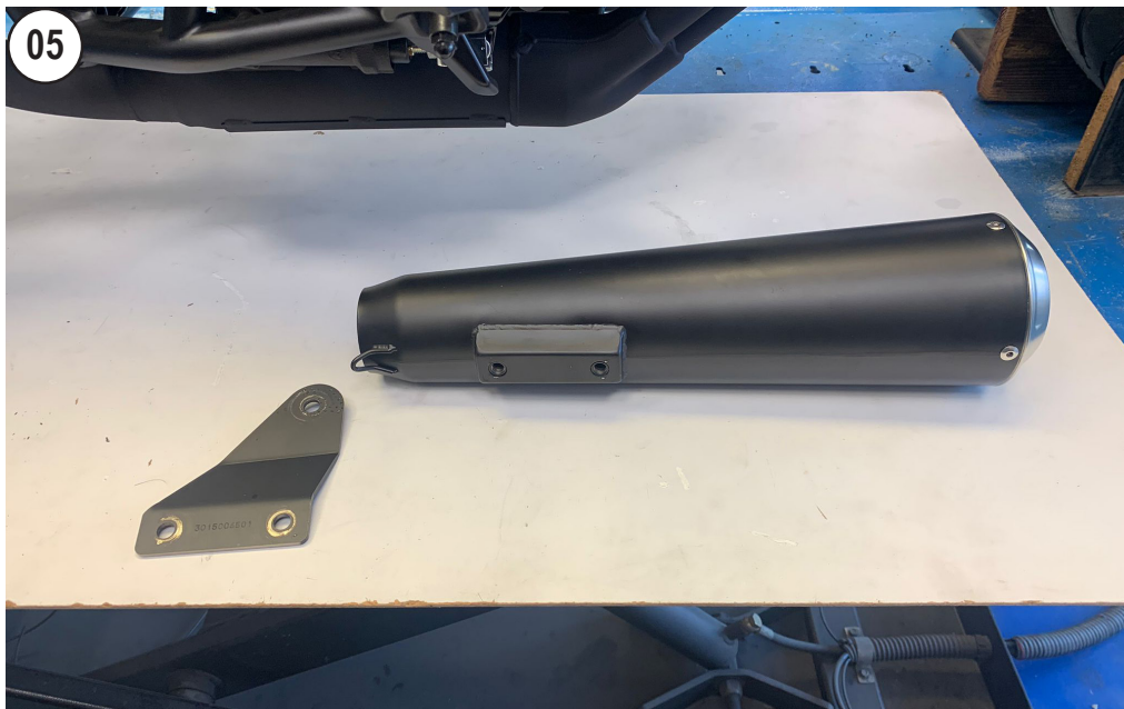
INSTALL THE BRACKET ON THE MUFFLER
