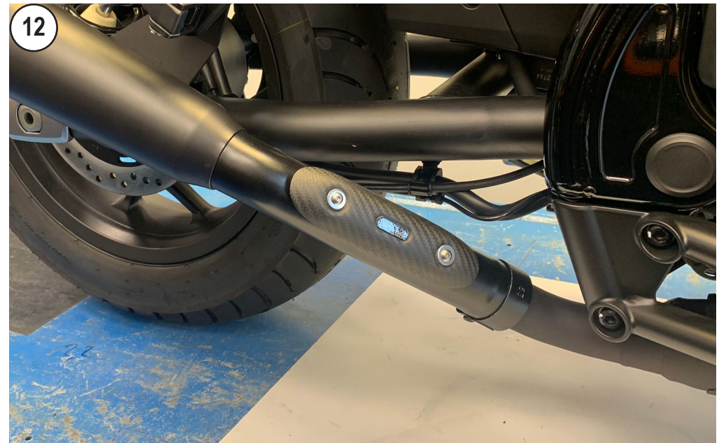
FIT THE CARBON HEAT SHIELD
