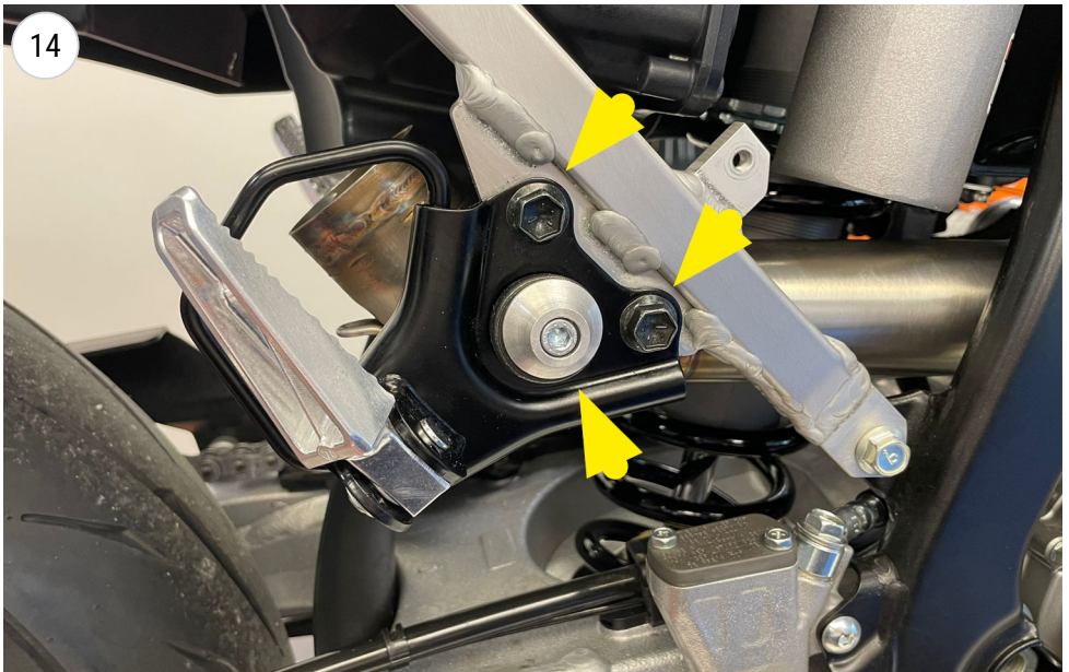
re-install the passenger's footboard and screw
