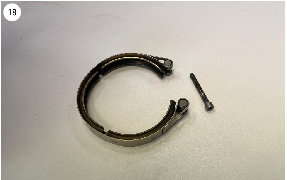
remove the screw from the clamp to allow assembly
