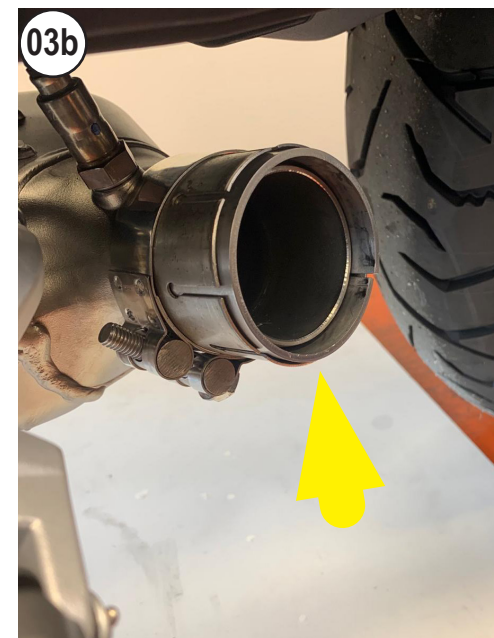
FIT THE S.S. BUSHING ON THE STOCK PIPE
