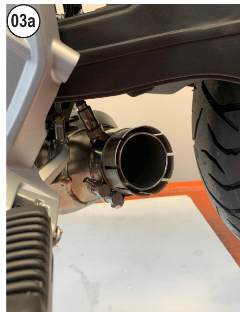
FIT THE S.S. BUSHING ON THE STOCK PIPE
