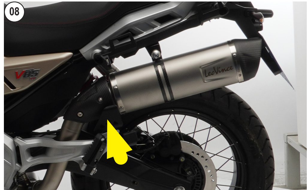
HANG THE SPRING AND INSTALL THE CARBON HEAT SHIELD
