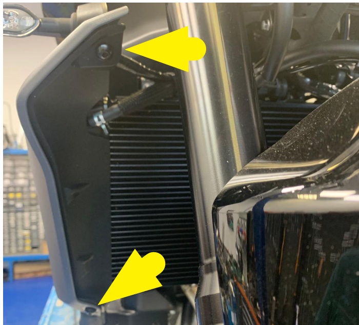
UNSCREW AND REMOVE THE FAIRING
