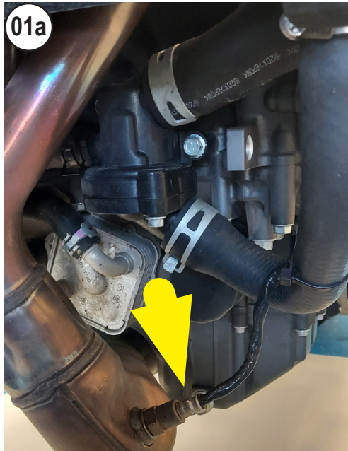
UNSCREW THE LAMBDA SENSOR
