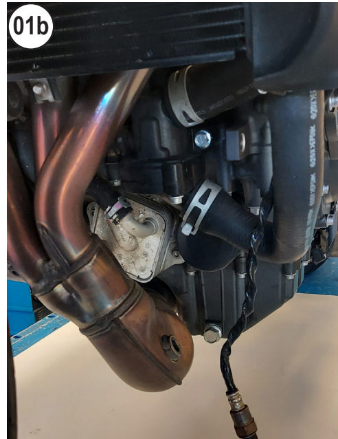
UNSCREW THE LAMBDA SENSOR
