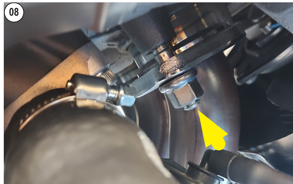
UNSCREW AND REMOVE THE STOCK PIPE
