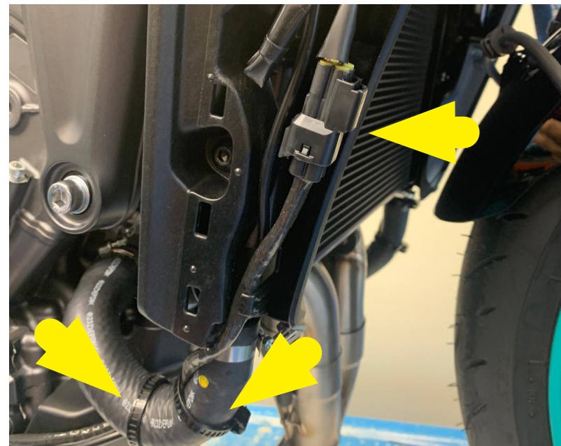
DISCONNECT THE STOCK CONNECTOR AND THE STOCK ZIP
