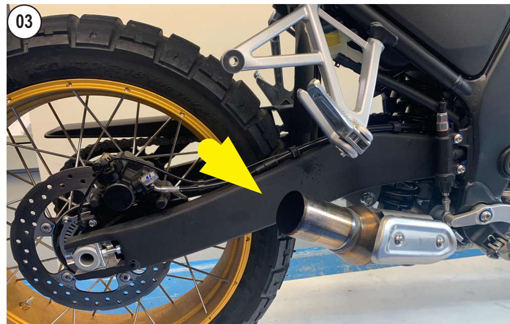
REMOVE THE STOCK MUFFLER
