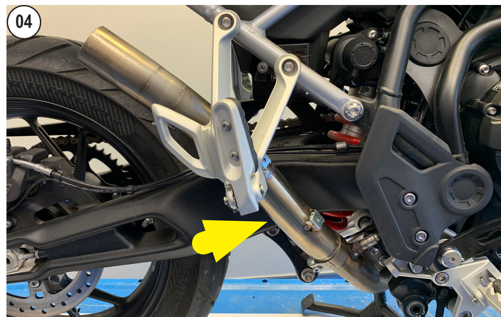
INSTALL THE LeoVince PIPE
