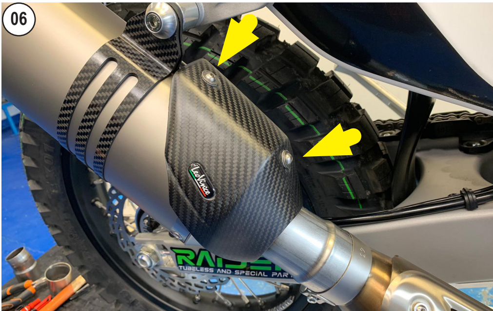
06 INSTALL THE CARBON HEAT SHIELD
