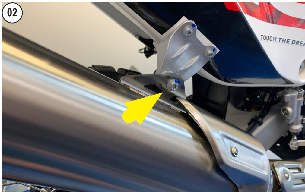
02 UNSCREW AND REMOVE THE STOCK SILENCER
