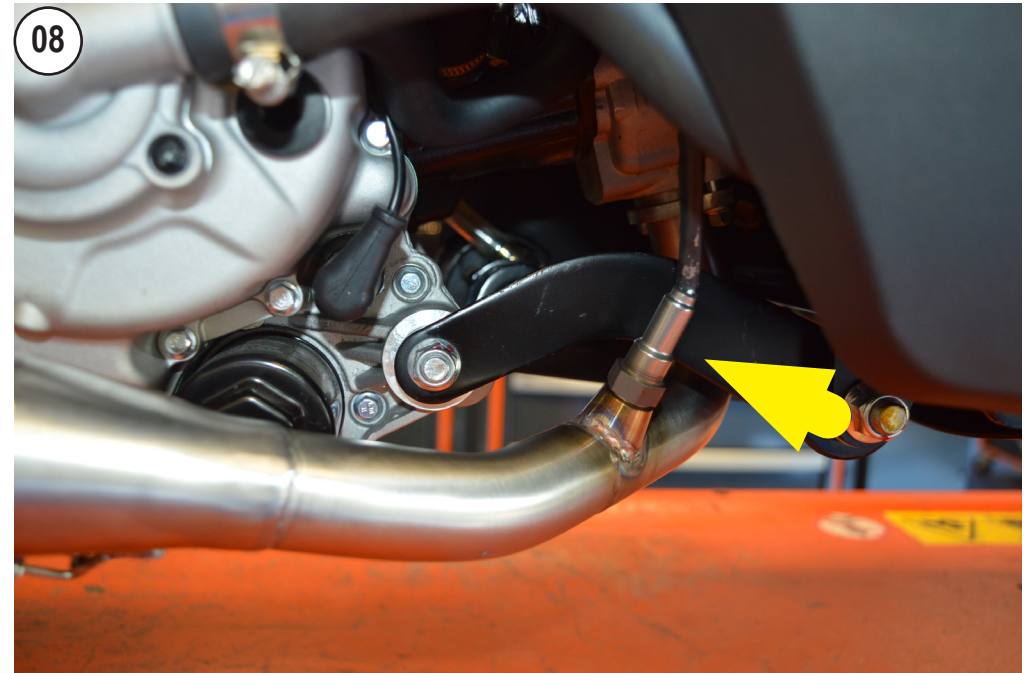
REINSTALL THE LAMBDA SENSOR
