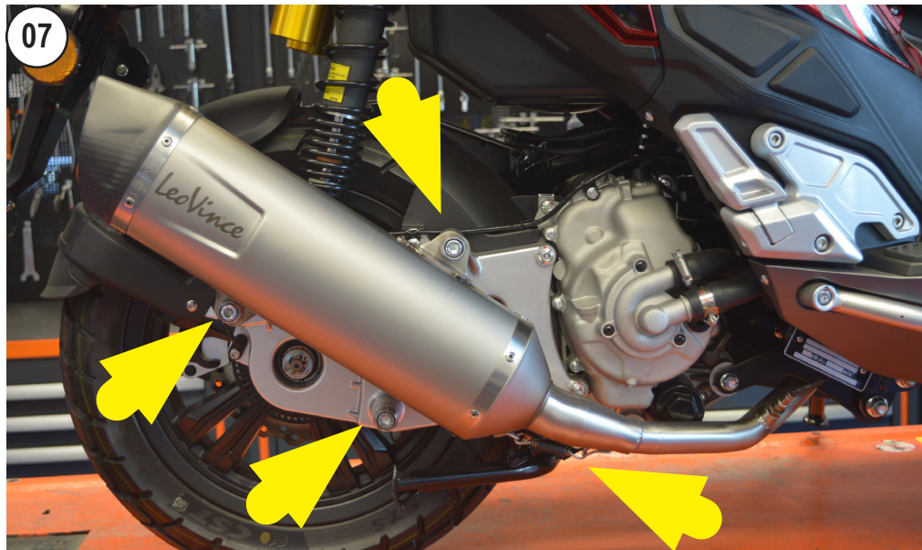
HOOK UP THE SPRING AND FIX THE SCREWS
