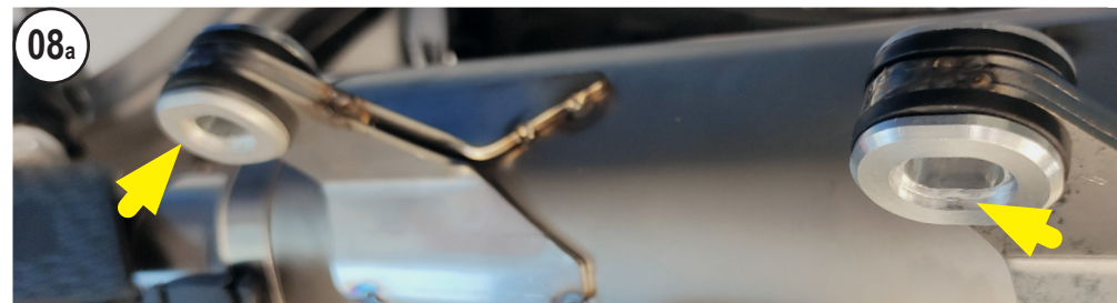
KTM/GASGAS - FRAME SIDE COLLAR WASHERS - P/N 207110
